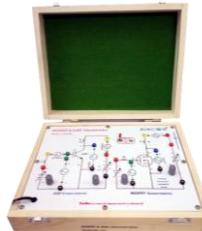
**SINCOM SA-121DM MOSFET & IGBT Characteristics** with Digital meters is comprehensive remarkable trainer useful to study V-I characteristics of MOSFET and N-Channel IGBT. The power MOSFET and IGBT are mainly used in switching circuits and power electronics applications. The trainer is simply designed to plot its characteristics and determine the various operational parameters in a simple experimental way. The trainer is equipped with on board Digital voltmeter and Digital Ammeter.
