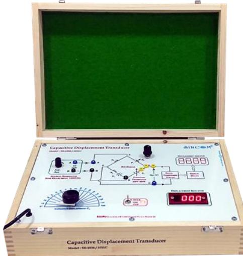
**SINCOM SE-1036 Capacitive Displacement Transducer** is an exceptional trainer designed for measuring Capacitive displacement using capacitive transducer. This comprehensive trainer comes with a 3<sup>1/2</sup> digit LED Displacement Indicator, allowing for precise and accurate measurements. It also features calibration control, AC excitation input control, and a marked capacitive displacement scale, making it easy to track and analyze displacement input.
